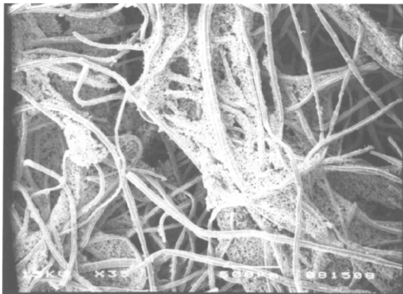
Fig. 1. SEM pictures of a 90% porous 'Fibrex'-sintered electrode substrate material.
